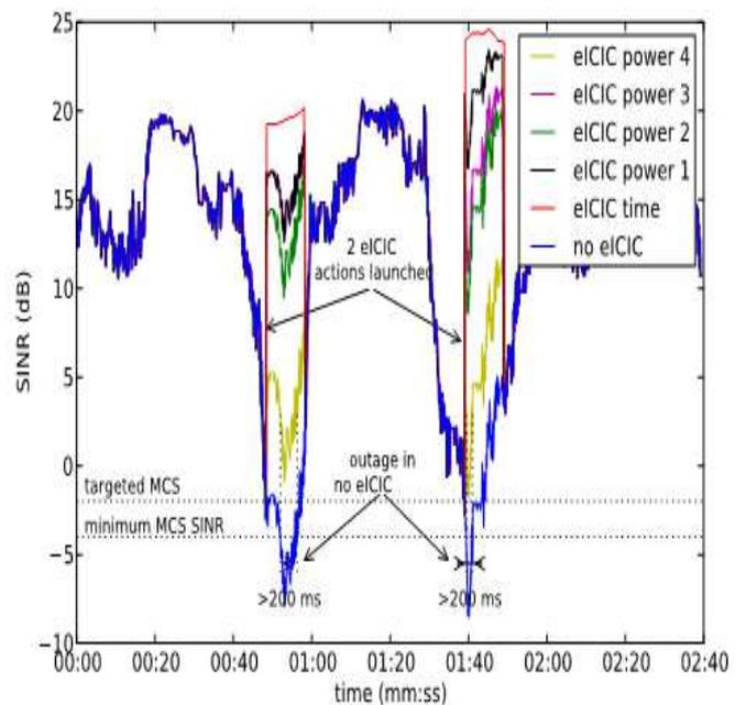
Fig. 3: SINR versus time of a victim MUE when passing close to two houses.
